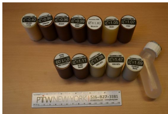
Figure 3.2: Gammex tissue equivalent materials used in the CT measurements. First row from left to right: Lung (LN-450), Adipose (AP6), Breast, CT Solid Water, Muscle, Brain, Liver LV1. Second row from left to right: Inner Bone, Bone B200, Bone CB2-30% Mineral, Bone CB2-50% Mineral, Cortical Bone SB3 and the true water bin.
