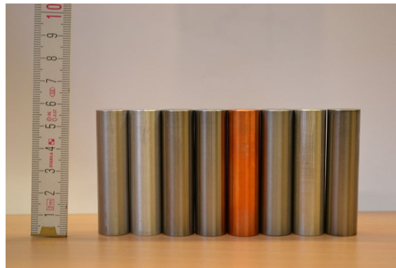
Figure 3.1: The metal rods used in the CT measurements. From left to right: MCP-96, aluminum, titanium, iron, copper, molybdenum, tin, tungsten.
