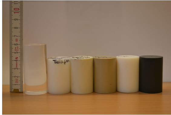
Figure 3.3: Polymers used in the CT measurements. From left to right: PMMA, Tecaform, Tecadur, Tecapeek, Teflon, PVC.
