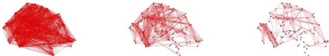
Fig. 2.2: Schematic of functional network visualization for increasing threshold values, Achard et al. [ASW + 06].
