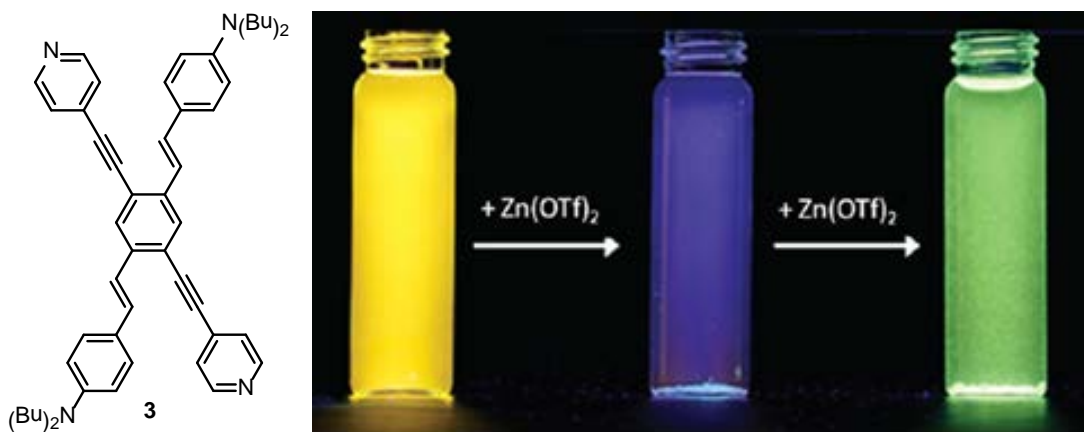
Figure 10 A picture showing the fluorescence response of cruciform 3 in chloroform (left), after addition of a small amount of zinc (middle), and after addition of an excess of zinc (right) (adapted from Acc. Chem. Res. 2010 , 43 , 397).
