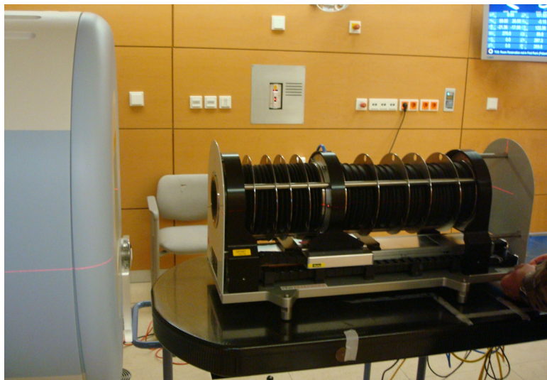
Figure 3.1. PeakFinder TM used for depth dose measurements positioned on the treatment table at HIT. The beam comes from the nozzle on the left side.
