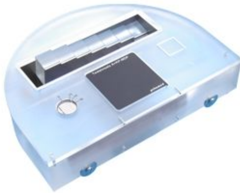
Figure 3.13: PEHA med test phantom for digital mammography (courtesy of DuMed).
