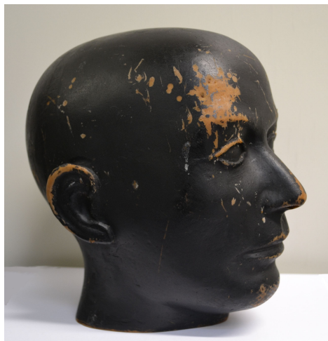
Figure 3.12: The anthropomorphic head phantom consists of a human skull surrounded and filled with tissue equivalent material.
