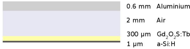
Figure 4.1: Detector geometry and composition as used for Monte Carlo simulation.
