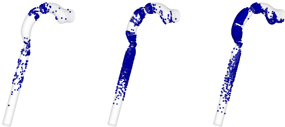
Fig. 5.26: Particle deposition pattern on the wall of cast-based mouth-throat at inspiration flow rate of 60 L/min for particle of 2 (left), 5 (center), and 10 (right) \mu\text{m} .
