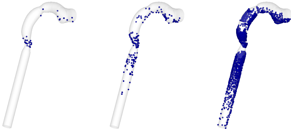
Fig. 5.25: Particle deposition pattern on the wall of cast-based mouth-throat at inspiration flow rate of 30 L/min for particle of 2 (left), 5 (center), and 10 (right) \mu\text{m} .
