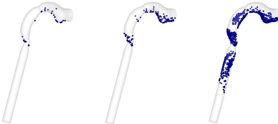
Fig. 5.24: Particle deposition pattern on the wall of cast-based mouth-throat at inspiration flow rate of 15 L/min for particle of 2 (left), 5 (center), and 10 (right) \mu\text{m} .
