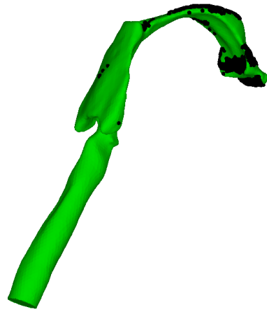
Fig. 5.107: The 10 \mu\text{m} particle deposition on the surface of the mouth-throat model of the CT-based mouth-throat.
