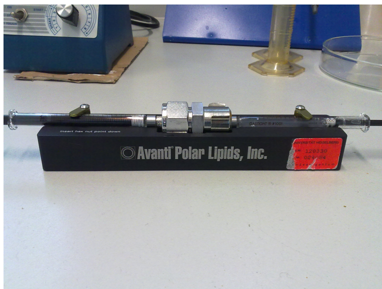
Figure 2.10: This manually operated extruder was used for the production of small unilamellar vesicles of about 100 nm size.
