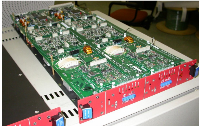
Figure 2.11: The inner structure of a A4601H Power Supply Module. Each module hosts two boards. Each board has 2 LV and 2 HV channels serving one power group of the tracker.
