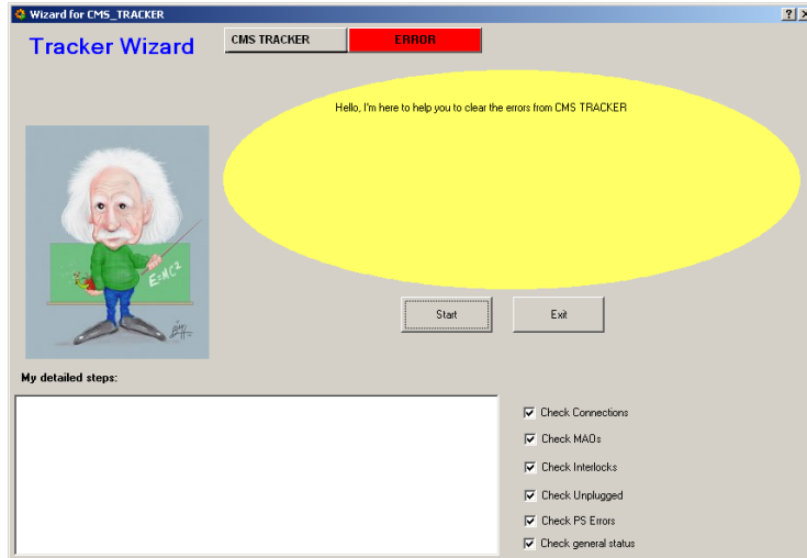
Figure 4.25: The user interface for the CMS Tracker Wizard, called on the CMS tracker top node. The user interaction is limited to two or three possible choices. The expert can choose to perform only some of the different kinds of checks.
