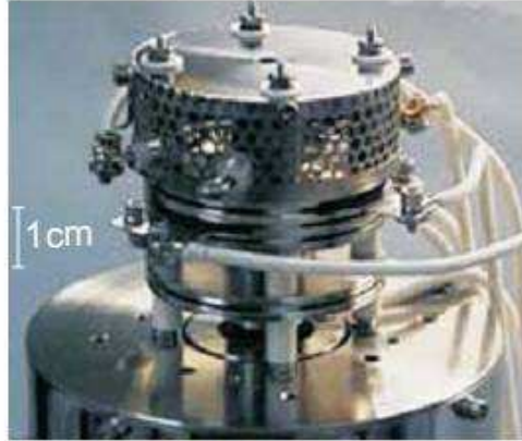
Figure 5.5: Electron impact ion source from ABB Extrel [58] for the ionization of atomic or molecular beams and gaseous species.
