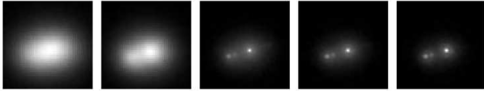
Figure 2.3: Lucky Imaging with AstraLux Sur. From left to right: (1) Sum of 50 000 images with 25 ms integration time in SDSS z' -band. (2) All 50 000 images, shifted on the brightest pixel in each image and added together. The resolution is seeing limited. (3) Best 50% of the images combined, selected by Strehl ratio. The seeing halo is dramatically reduced. (4) Best 10% combined. (5) Best 1% combined. The resolution is almost diffraction limited and the closely separated secondary and tertiary star are clearly resolved. Taken from Hippler et al. (2009).
