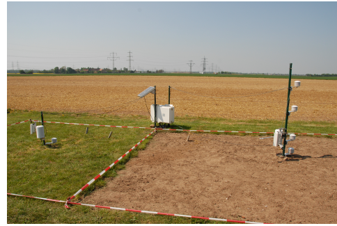
(b) Field experiment under grass and a bare surface. The stakes mark the position of the soil profiles. Relative humidity, air and surface temperature are measured directly above the corresponding surface cover.
