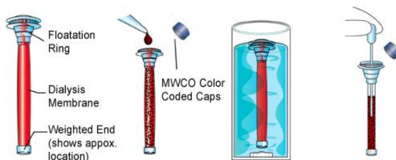
Figure 4.1.2. The figure shows different parts of the cellulose ester membrane dialyser and displays different steps involved from the sample addition to the color coded membrane dialyser, dialysis technique and sample recovery after dialysis respectively.
