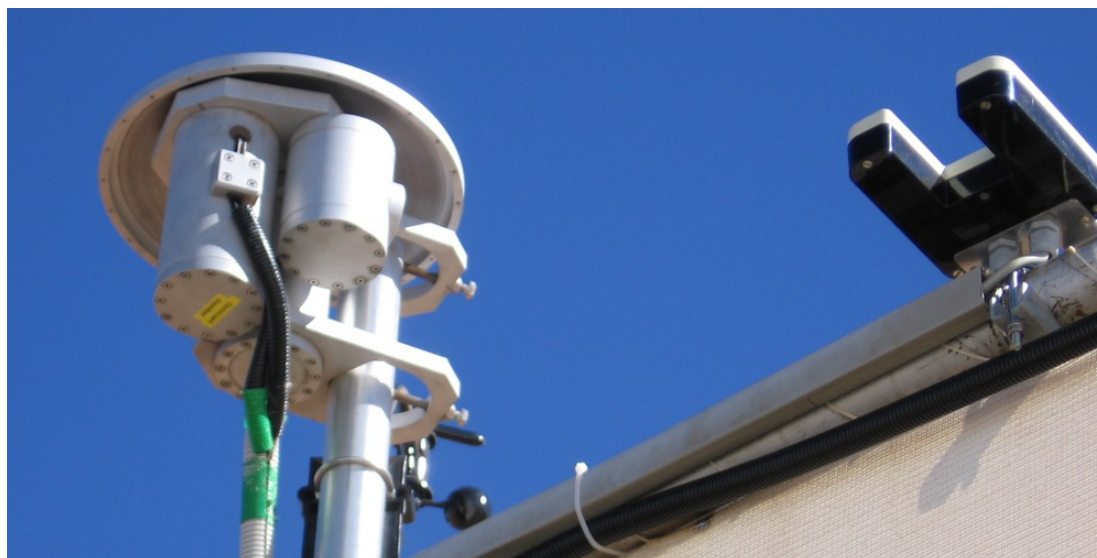
Figure 2.15.: top : HTML interface to cloud monitor measurements. The bright spot visible in the right hand panel is the moon. bottom : photo of the sky monitor device and the rain sensor, mounted next to the ATOM building.
