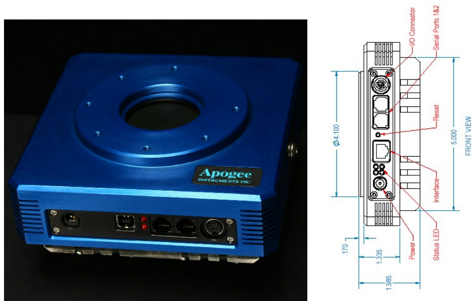
Figure 2.7.: ATOMs main CCD camera (image credit: Apogee Imaging Systems )
