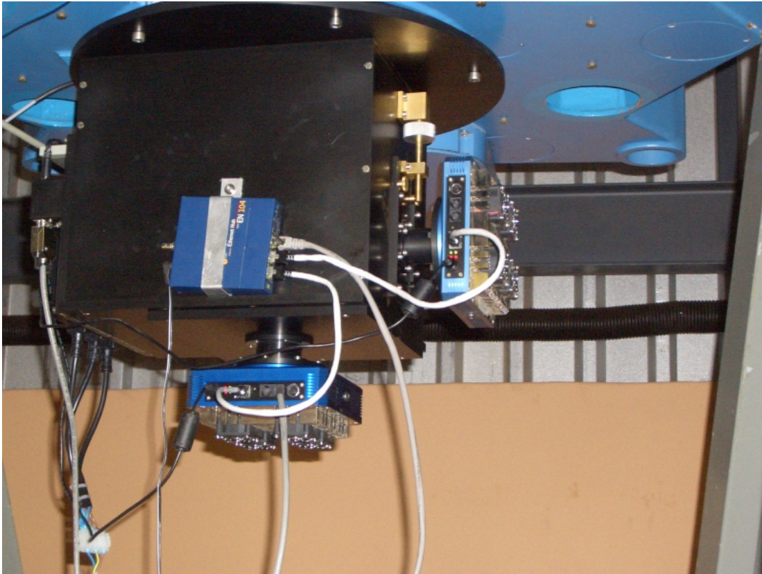
Figure 2.6.: Instrument below the mirror cell: Main camera is at the bottom, the guiding camera to the right. The device in the front is a small Ethernet hub which distributes the control signals to/from the cameras. The control cable of the filter wheel unit can be seen at the left. It is connected to the RS-232 port of the guiding camera, which acts as a signal/media converter to tunnel the signals from the control computer via Ethernet to the filter wheel unit.
