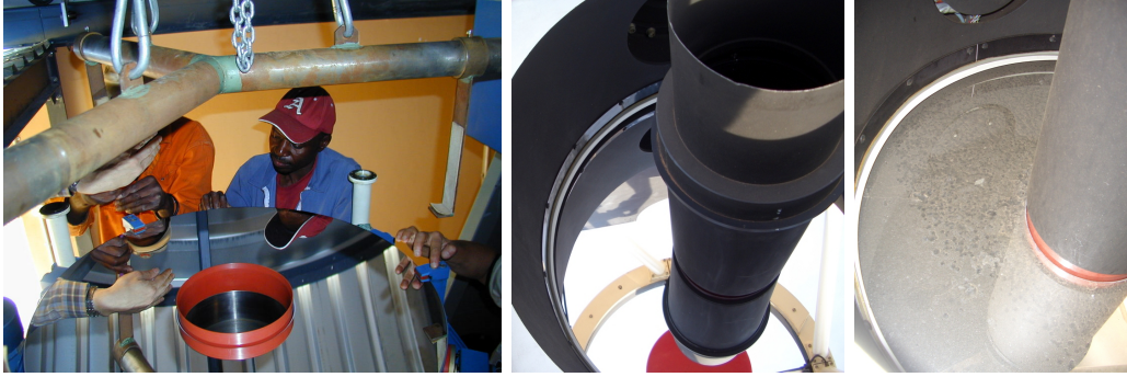
Figure 6.3.: A macroscopic view on the mirror degradation by dust. From left to right: during installation (Aug 2005), after a few month in Namibia in Nov 2005 and four years later in Nov 2009.
