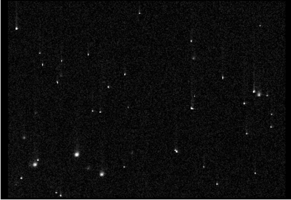
Figure 2.3: Cutout from of the 0.4s F555W-band image to display the effect of the CTE problem. Stripes along the y-axis demonstrate the loss of charge during the readout. The displayed area is selected from a region on the detector with large y-coordinates to highlight the effect.
