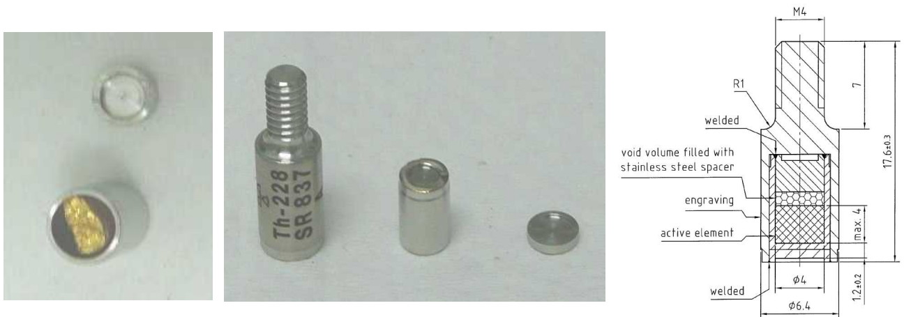
Figure 67: Photos of the inclusion of the radioactive gold foil into the double encapsulation of the Borexino ^{228}\text{Th} source. The profile of the encapsulation is shown on the right, the lengths are given in millimeters. (Images courtesy of Eckert und Ziegler Nuclitec GmbH)
