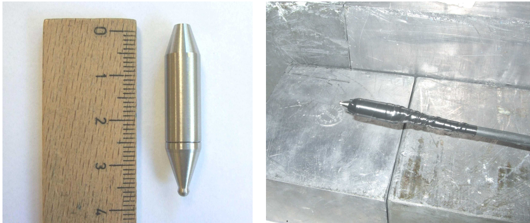
Figure 70: Representation of the source holder used for the ^{228}\text{Th} source during the first external calibration campaign in Borexino. The source holder is made of stainless steel and was welded with a fish tape. The picture on the right shows the source holder after embedding of the ^{228}\text{Th} source and before the first insertion into the detector (July 5, 2010). Adhesive foil was used to fix the screw of the source holder.
