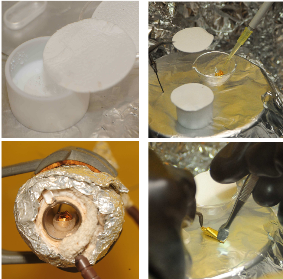
Figure 66: Production of the Borexino ^{228}\text{Th} source (from left, top, to right bottom): Conversion of \text{ThCl}_4 into \text{Th}(\text{NO}_3)_4 ; Transfer of \text{Th}(\text{NO}_3)_4 into gold crucible; Conversion of \text{Th}(\text{NO}_3)_4 into \text{ThO}_2 ; Insertion of gold crucible into gold cover.
