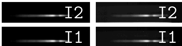
Figure 4.12: Coherent averaged images. Left the real and right the imaginary parts of the coherently averaged image for each interferometric channel.
