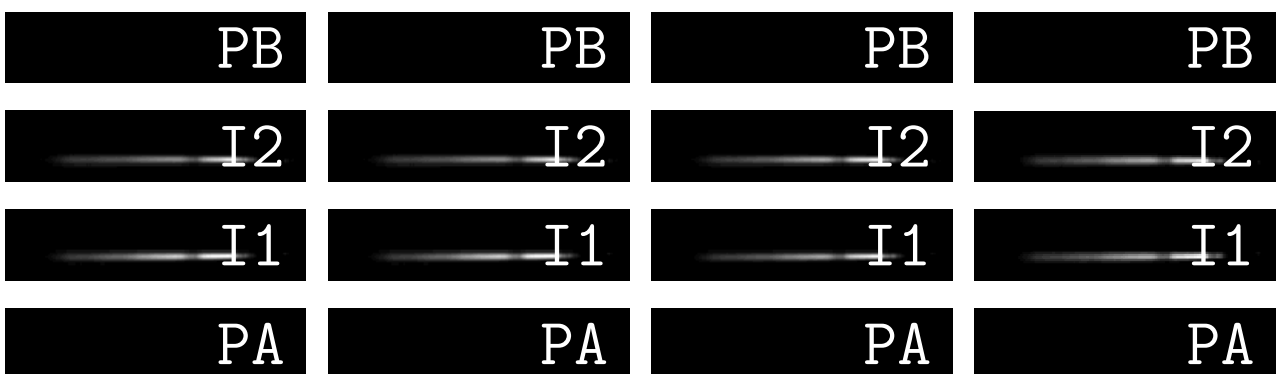
Figure 4.10: The first and second column show the predicted photometry I_{2A} , I_{1A} and I_{2B} , I_{1B} in the two interferometric channels in the middle, respectively. The third column gives an estimate of the photometric fluxes I_{1A}+I_{1B} and I_{2A}+I_{2B} in the interferometric channels, while the fourth column gives the geometric mean images \sqrt{I_{1A}I_{1B}} and \sqrt{I_{2A}I_{2B}} (uncorrelated fluxes).
