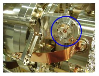
Figure 3.9: A sample 2 K thermal anchor (circled in blue) for the HV electrode cables plus Cu cooling bands between the Cu cooling unit on the right and a neighbouring vacuum chamber in the bottom left corner.
