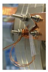
Figure 3.12: Silicon diode sensor and its thermally anchored cables.
