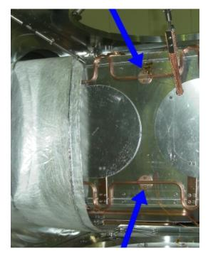
Figure 3.10: Photo of the 80 K thermal shields with water cooling lines (contact points with the shield are marked with arrows) and multilayer insulation (on the left) visible. A braided copper wire used to thermally anchor one of the chamber suspension wires is visible in the upper right corner. Two access ports to the enclosed 40 K shields and vacuum chambers can also be seen.
