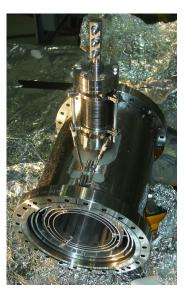
Figure 3.19: Photo of the bake-able, charcoal-based, UHV cryopump.
