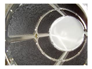
Figure 3.18: Activated charcoal layer of the cryopump.
