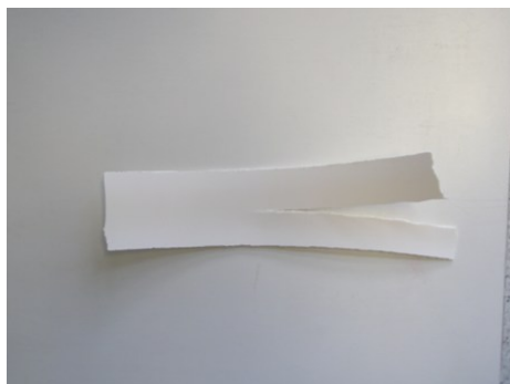
Figure 83. Ribbon split up in two halves obtained after roller-compacting a blend of MCC with 12.5% water addition.
