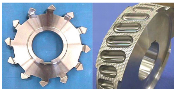
Figure 11. Rotor designs commercialized by Gerteis. Star (left) and pocketed rotor (right)
