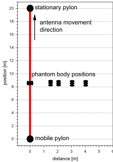
Figure 2.2.: Test arrangement for the footprint analysis. The black dots visualize the phantom body positions orthogonal and parallel to the radar line.
