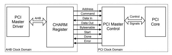
Figure 6.2: Communication flow of the PCI Master driver.
