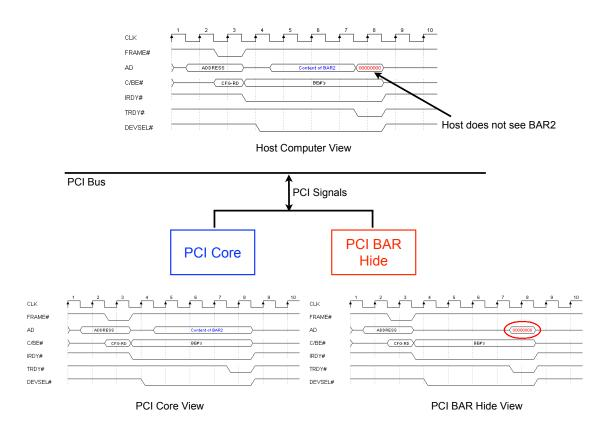
Figure 4.6: PCI Configuration Space hiding.
