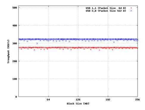
Figure 9.7: Read throughput to the CHARM USB CD-ROM device corresponding to the block size of the transfer. The color of the bars defines one of the USB packet sizes of the device: USB 1.1 (64 B) or USB 2.0 (512 B).
