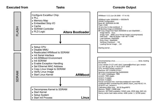
Figure 3.1: Boot process of the CHARM. First, the boot loader is executed from flash. Afterwards, the boot code is copied to the SDRAM and is started from the RAM. The console output of the CHARM is shown on the right side of the picture.
