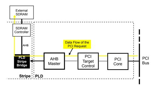
Figure 4.7: Layout of the PCI processing units.
