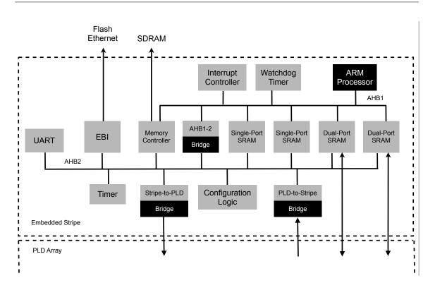
Figure 2.2: Structure of the Excalibur Embedded Processor Stripe [1].
