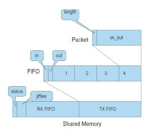
Figure 8.7: Layout of the shared SRAM content [3]. The left side represents the lower addresses. The right side marks the end of the SRAM content.
