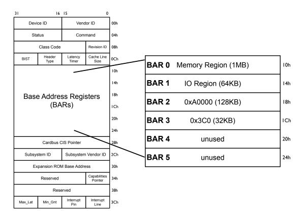
Figure 4.5: PCI Configuration Space of the CHARM.
