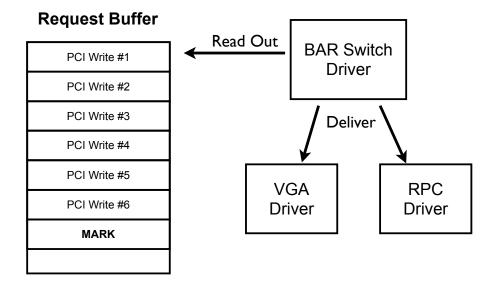
Figure 4.13: Processing of the Request Buffer. The BAR Switch driver reads out the content and distribute the data to the processing drivers.
