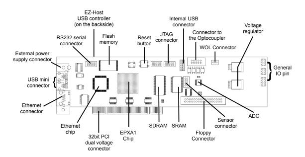
Figure 2.1: Layout of the CHARM board.
