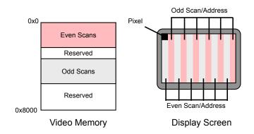
Figure 4.4: The screen is divided into odd and even columns.
