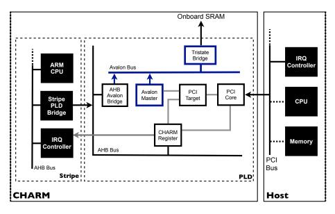
Figure 8.6: Block diagram of the network function of the CHARM.
