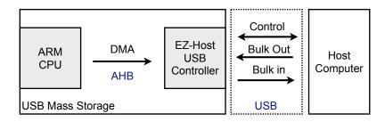
Figure 5.4: Overview of the processing units while mass storage emulation.
