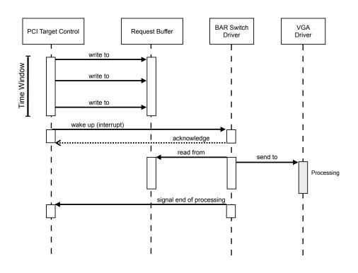
Figure 4.11: Timing of the access to the Request Buffer.
