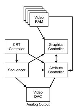
Figure 4.1: Diagram of the VGA data processing. The arrows describes the data flow.
