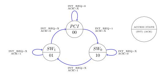
Figure 4.12: Request Buffer access synchronization.
