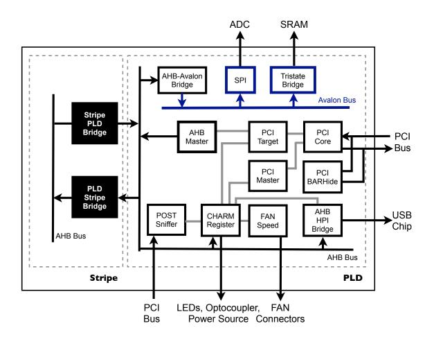
Figure 2.3: Structure of the CHARM PLD design.
