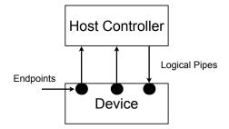
Figure 5.1: USB logical pipes.
