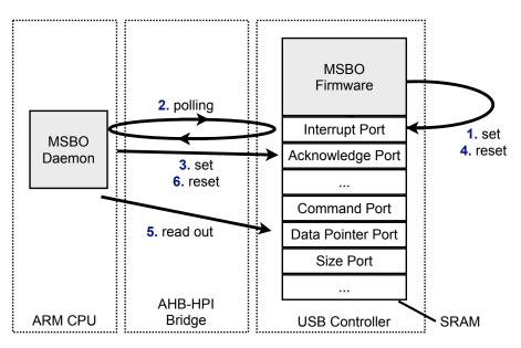
After the daemon detects an active interrupt, it acknowledges the request. Figure 5.6 illustrates the process of this protocol.
