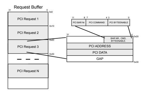
Figure 4.8: Structure of the Request Buffer
