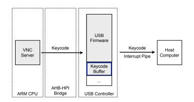
Figure 5.3: USB keyboard implementation. The VNC server takes the user interaction and converts it to USB keycodes. These keycodes are written into the keycode buffer inside the USB controller.
