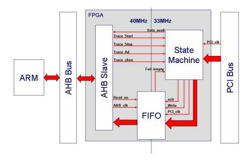
Figure 8.1: Layout of the PCI bus analyzer design [2].
