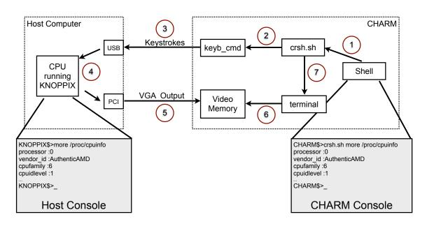
Figure 7.1: Functional overview of the crsh.sh program. The red circles define the processing order of the function units. On the right hand of the picture, a shell console calling the crsh.sh program is shown. The left side of the picture shows the screen content of the host computer.
