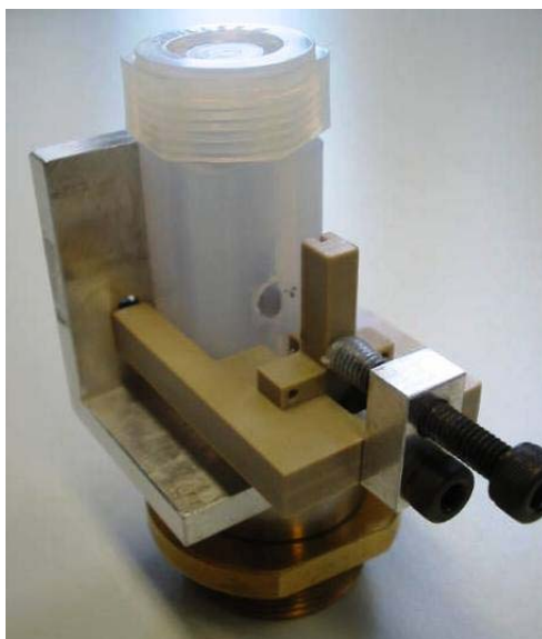
Figure 2.4 The home made sample holder and the measuring cell (R2)
