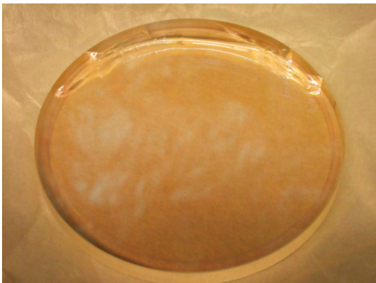
Figure B.1: A broken window after a bake-out at 125 °C. The crack along the top-half of the window is clearly visible.
