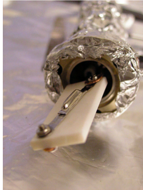
Figure 10.1: Two mounted NiCr boats as K dispenser. The white ceramic separator assure that the dispensers are not touching the vacuum chamber.
