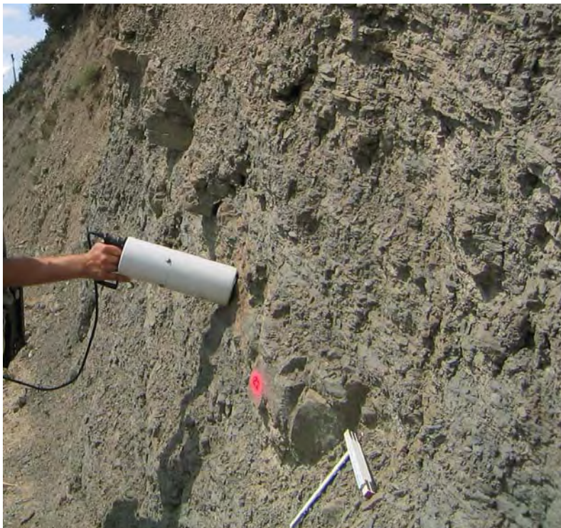
Fig. 3.8: Portable gamma ray spectrometer ( GR-320 enviSpec ) as used for outcrop measurements (section Latás, Spain).
