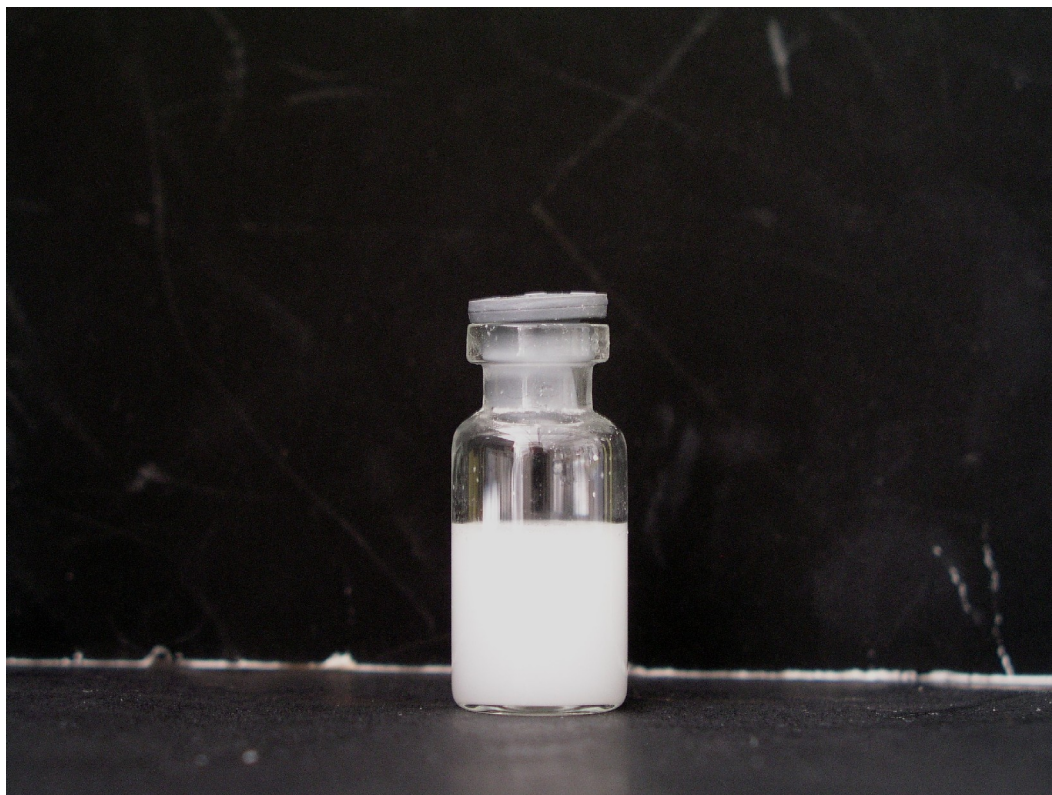
Figure 39: Image of a reconstituted lyophilizate of a CSA/CD formulation. Reconstituted by adding 2 ml and manual shaking. Image taken 1 day after lyophilization.
