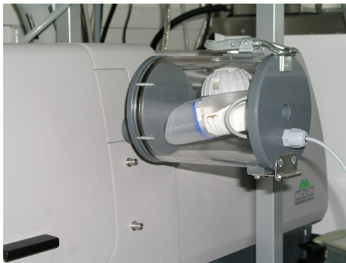
Figure 3: Detailed view of the nebulisation chamber containing the eflow®.
