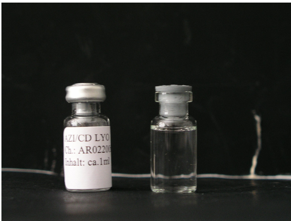
Figure 17: Image of a reconstituted lyophilizate of an azithromycin/cyclodextrin formulation. Reconstitution was made by adding 3 ml and manually shaking the vial. Image taken 1 day after lyophilization.
