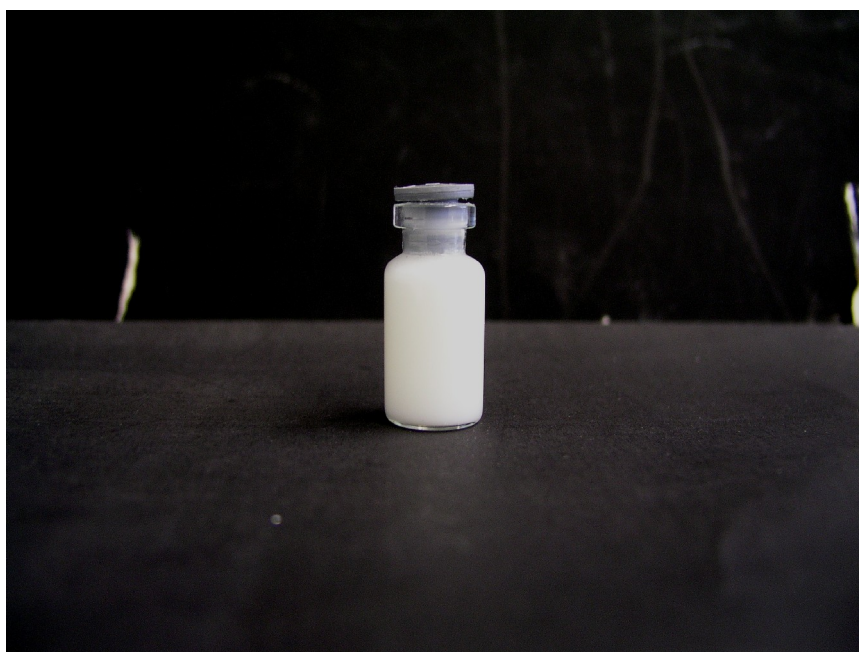
Figure 36: Image of a reconstituted lyophilizate of a CSA/CD formulation. Reconstitution was made by adding 3 ml and manually shaking the vial. Image taken 6 days after lyophilization.
