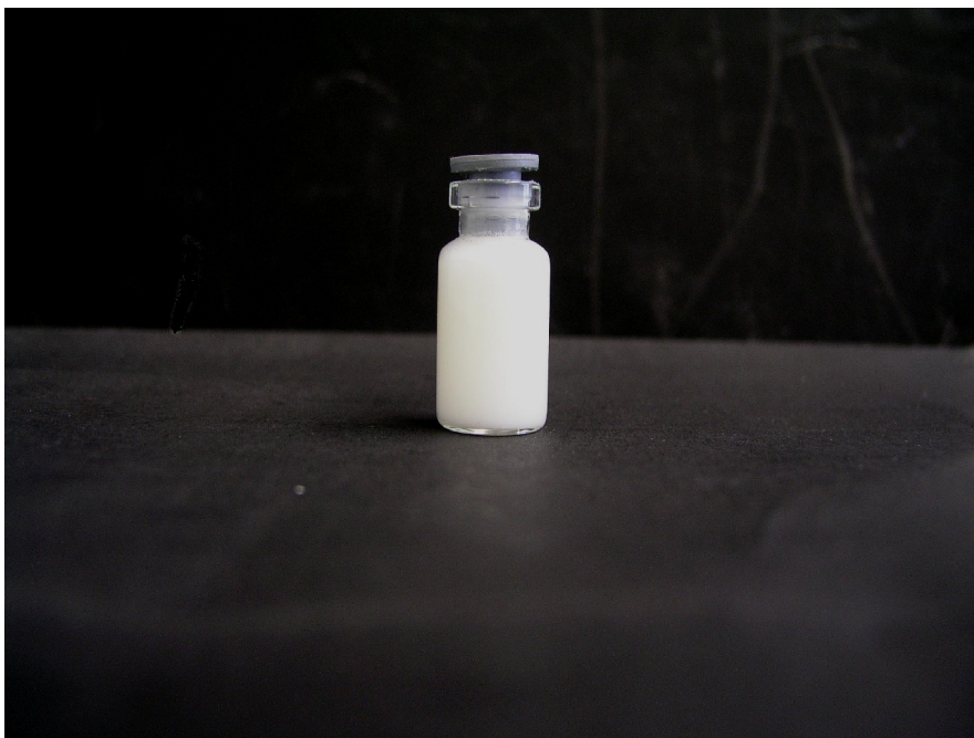
Figure 37: Reconstituted lyophilizate of a CSA/CD formulation. Reconstitution was performed by adding 3 ml and manually shaking the vial. Image taken 1.5 months after lyophilization.
