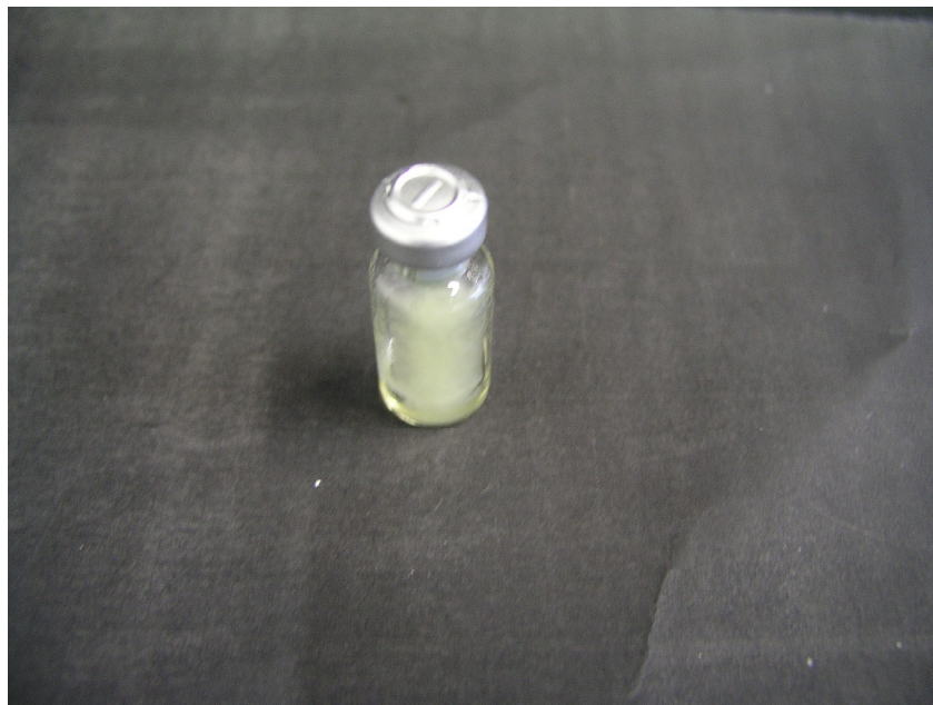
Figure 35: Image of a lyophilizate of a CSA/CD formulation. Image taken 6 days after lyophilization.
