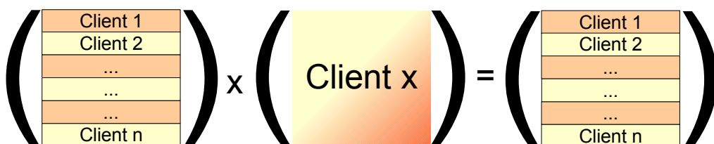
Figure 3.9: Data accessed by the clients, entries are read from matrix A and B and written to matrix C
