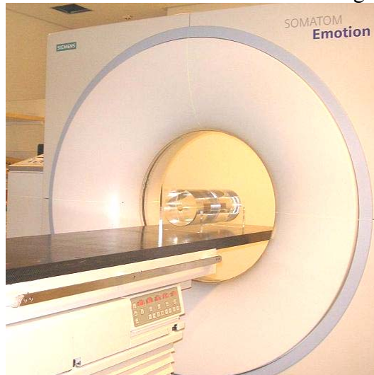
Figure 22. Emotion CT scanner with the PMMA phantom, positioned for CT-value measurements.
