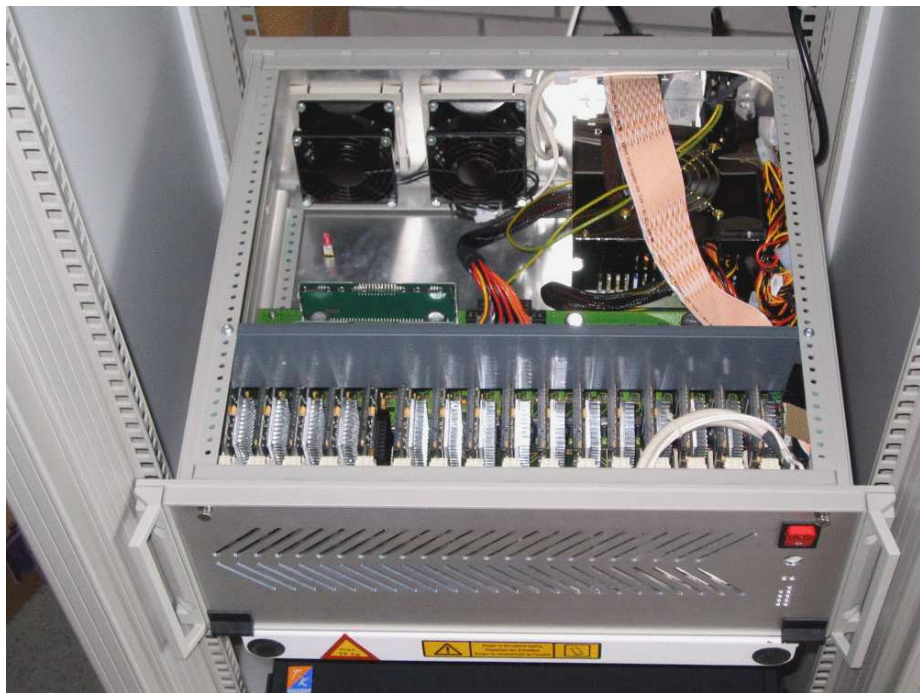
Figure 2.13: The distributed system with 16 network modules mounted on a backplane in a 19" rack. For the experiments presented in this thesis, a different system with only a single HAGEN chip was used.
