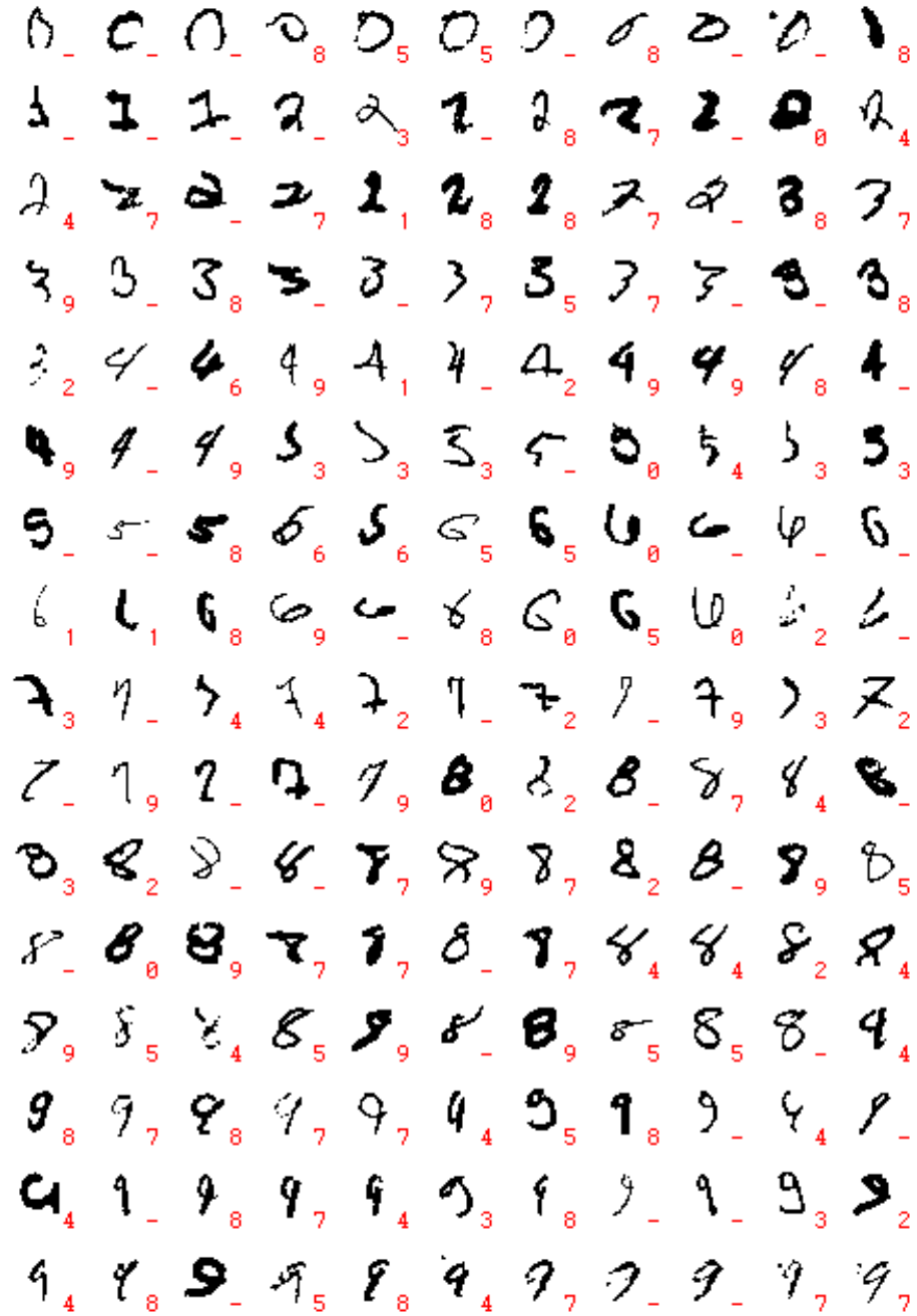
Figure 4.5: All 176 (out of 10,000) misclassified test images for one selected training run. Small numbers show the class predicted by the neural network. A dash (-) indicates that two or more classes received an equal voting count.
