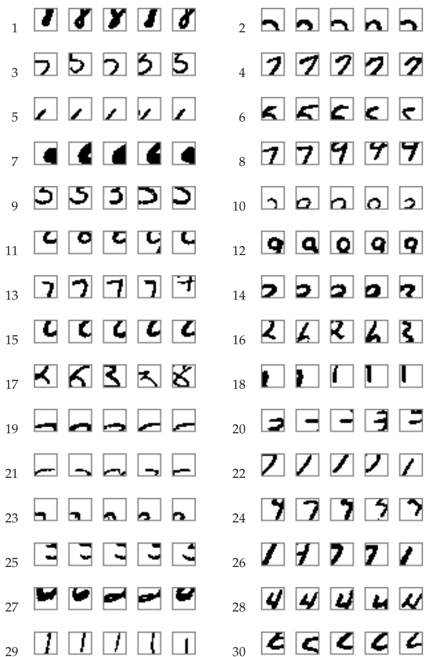
Figure 4.4: Detected features in layer S2 after self-organization (MNIST experiment) for 30 selected neurons (of 150 total), five strongly activating receptive field stimuli are shown. Neurons taken from the same network as in Figure 4.3
