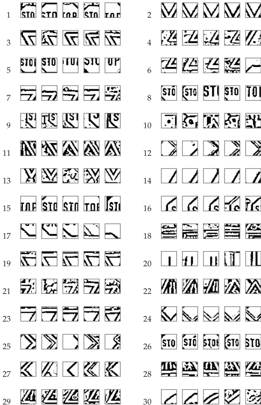
Figure 4.8: Detected features in layer S2 after self-organization (traffic sign experiment). For 30 selected neurons (of 100 total), five strongly activating receptive field stimuli are shown. Same network as in Figure 4.7
