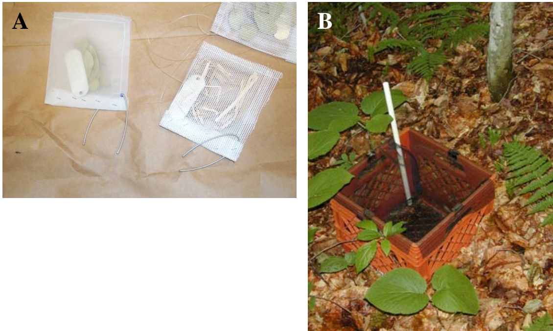
Fig. 39. Typical decomposition apparatus: A) Litter bag, B) Litter basket.
