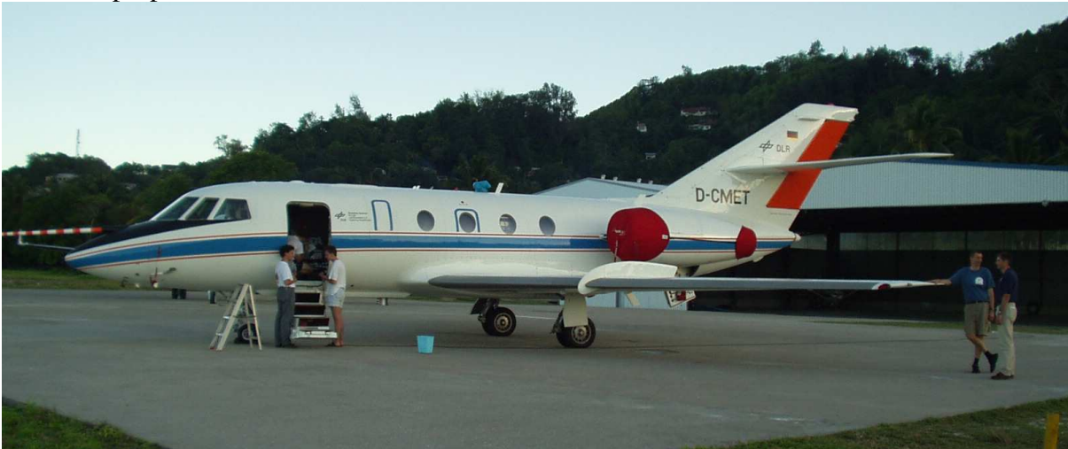
Figure 5-28: Photo of the Falcon on the airport in Mahé. When the plain is outside the hangar for longer periods, the upper housing has to be protected from rain (blue plastic bag). The lower housing is visible next to the stairway. (Also the Falcon is not waterproof – the blue basket stood inside for this purpose)
