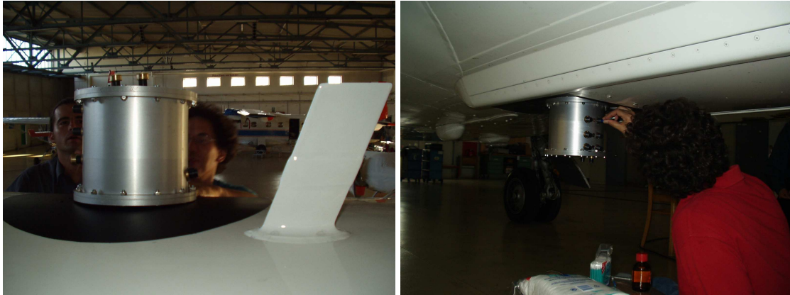
Figure 5-32: The housings installed on the Falcon. Left photo: upward direction and right photo: downward direction. Due to dirt raised by the front wheel, the downward telescopes must be cleaned with alcohol from time to time (right picture).
