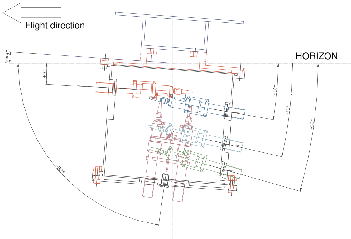
Figure 5-35: Figure of the lower dome as it was turned in the first FORMAT campaign. An average pitch angle of 4^\circ was observed in the campaign.
