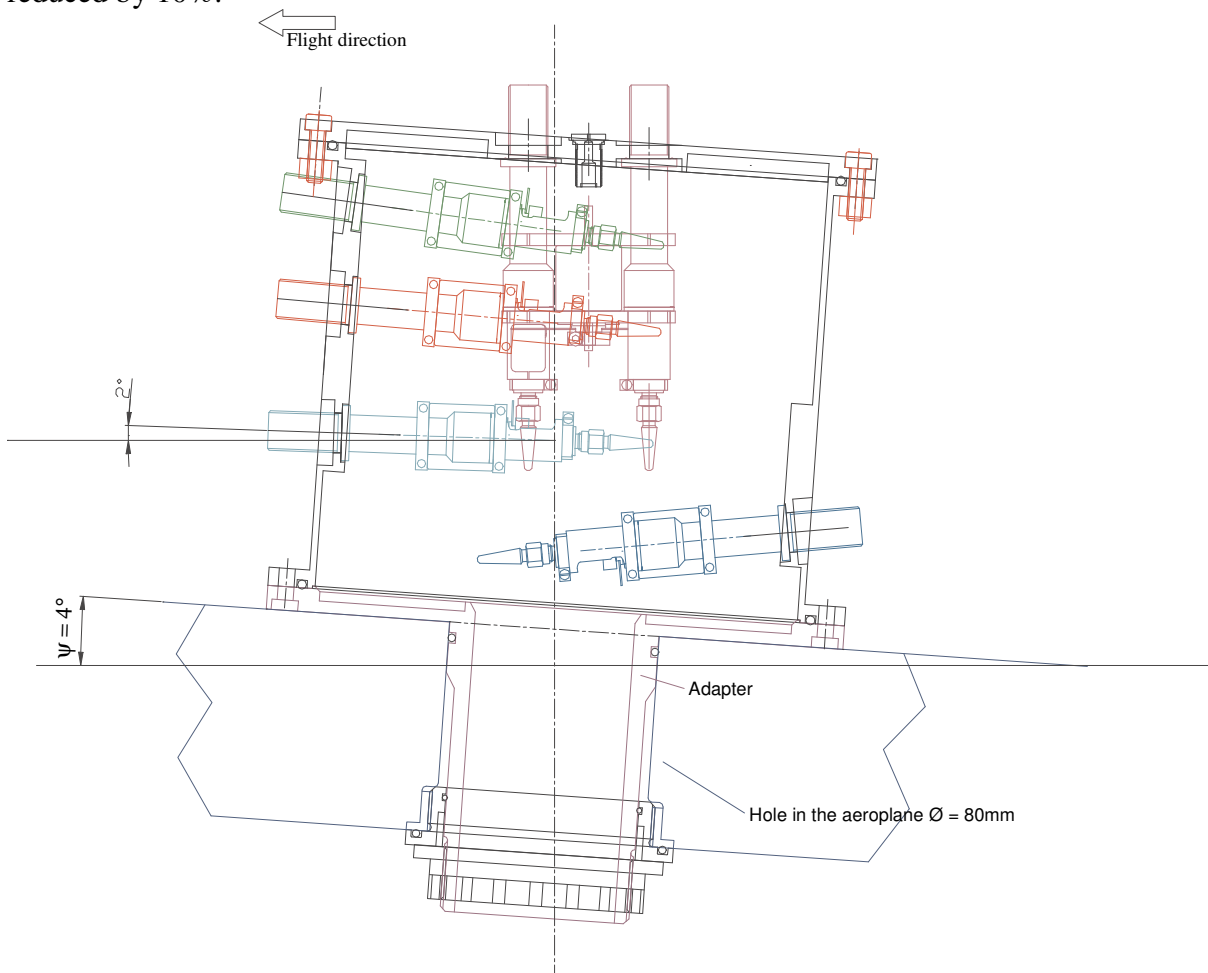
Figure 5-31: Detailed plan of the upper telescope housing (compare to Figure 5-4). Here the situation on the Falcon is shown.
