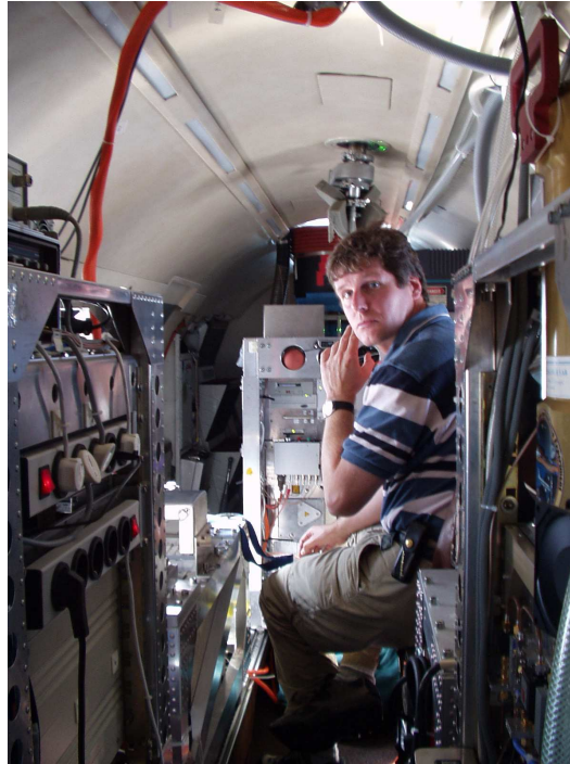
Figure 5-30: Photo taken inside the Falcon during one flight. The two large racks on the right and the left in the front of the picture belong to the ASUR, on the left in front of the ASUR the AMAXDOAS measurement rack is visible. The OLEX Rack is the one in the background of the picture behind its operator Andreas Fix.
