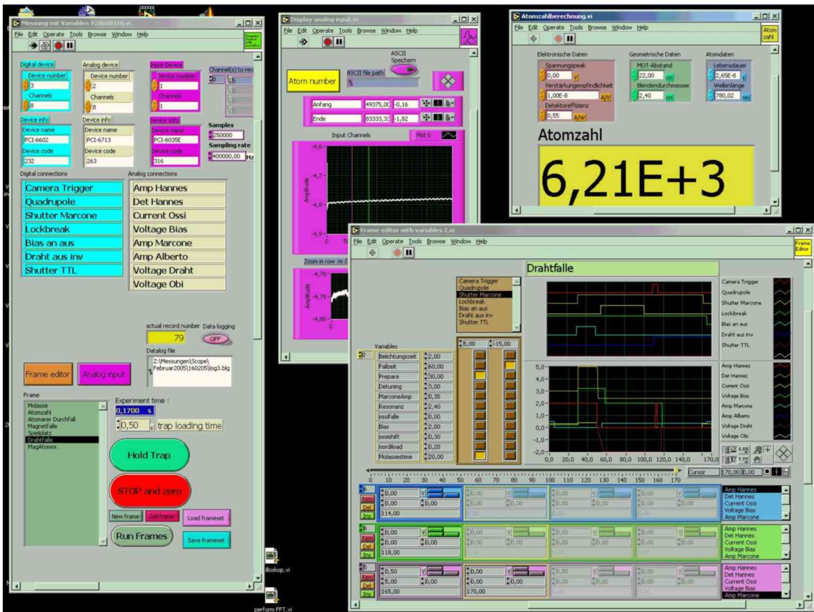
Figure 4.16: LabVIEW operation platform: The window to the left, contains all global parameters and allows to save and load settings and acquired data, the central window shows an input channel , which is analyzed in the window to the upper right to calculate the atom number from the fluorescence signal. The window to the lower right allows to edit the analog and digital output sequences.
