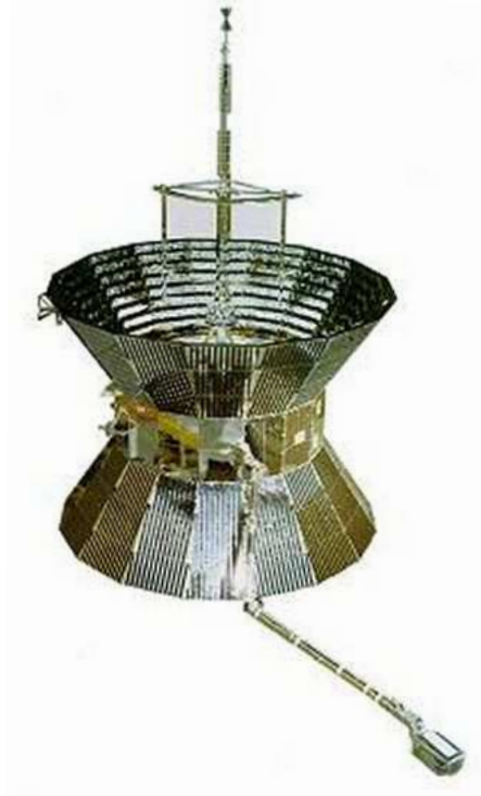
Figure 4.22: Picture of the Helios spacecraft. Note the cylindrical shape. Helios was stabilized in rotation around its antenna axis, directed along the main axis of the cylinder and pointing to the ecliptic north direction. The solar arrays are distributed all around the spacecraft body. The magnetometer boom in the bottom performed measurements of the IMF.
