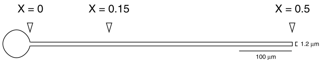
Fig. 2.1. Equivalent cylinder model (soma not to scale), with electrotonic length L = 0.5 . The locations of three synapses on the cable (electrotonic location X = 0, 0.15 and 0.5 ) are indicated by arrows.
