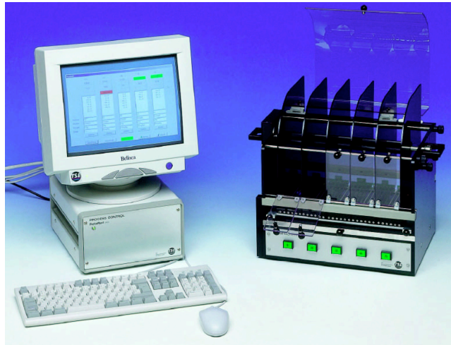
Figure 29 TSE Rota Rod apparatus for analysis motor coordination and balance and motor learning.
