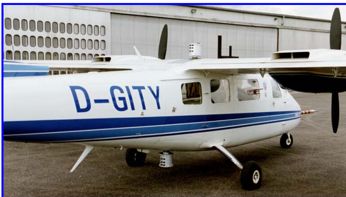
Figure 10.1.1 Partenavia aircraft with the AMAX DOAS instrument fitted to it. The telescope housings can be seen on top and bottom of the hull [Heue et al. 2001].
