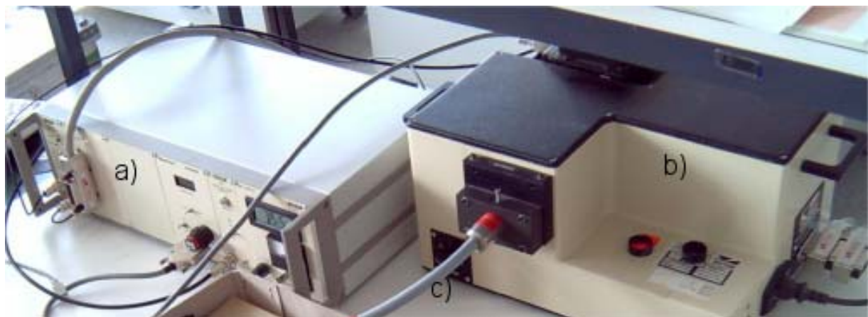
Figure 12.2.2 assembled spectro radiometer: a) electronics module, b) double monochromator, c) quartz fibre bundle
