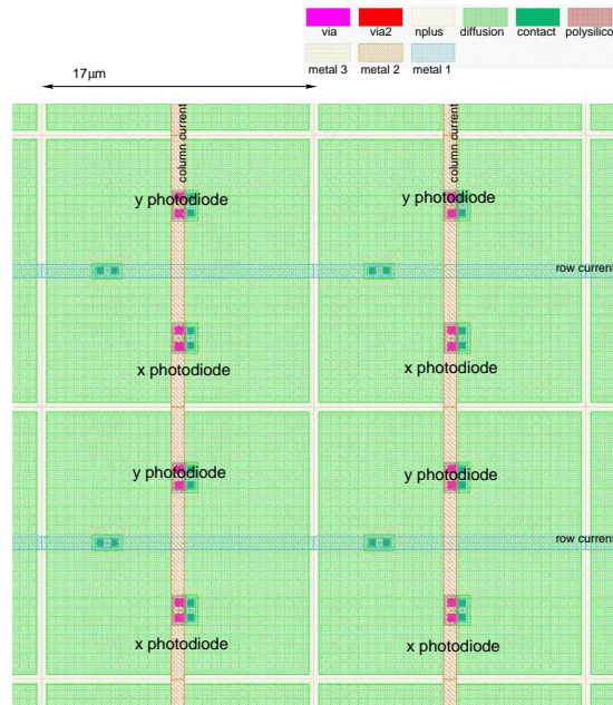
Figure 4.21: Layout of the prototype's pixel array. Each pixel contains two n+ /substrate photodiodes.
