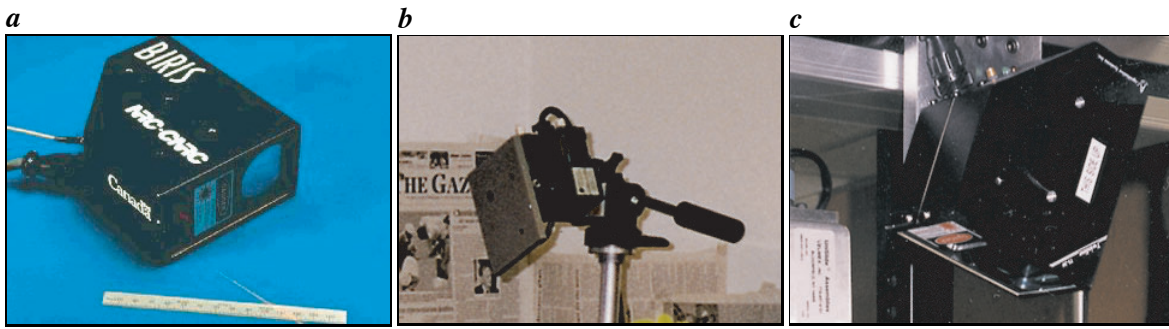
Figure 7.1: Biris range sensor: a sensor head, b pan-tilt unit and c mounted on a linear positioner.
