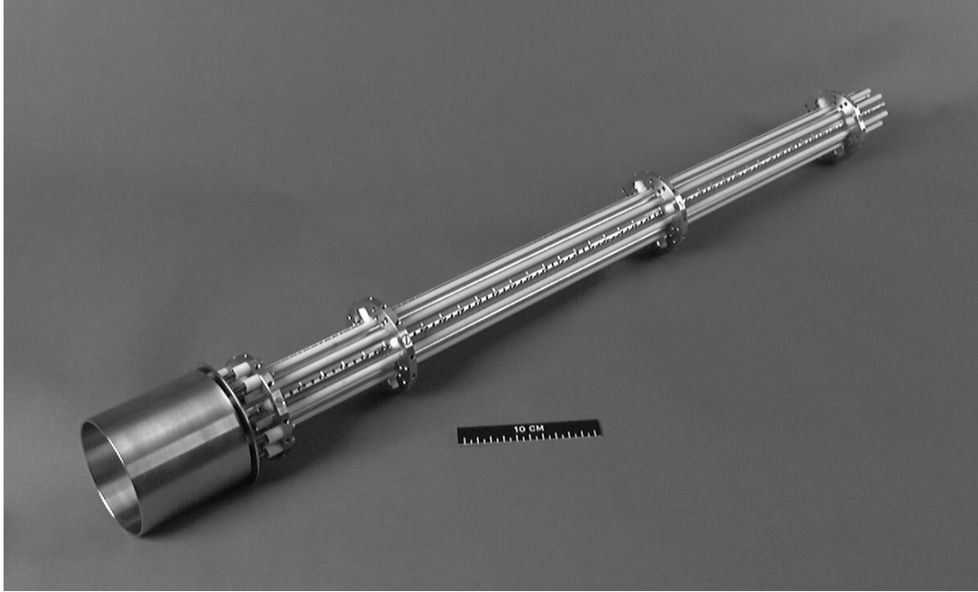
Figure 3.12: Photograph of the assembled four-rod electrode system of the ISOLTRAP ion beam cooler and buncher and the mounted deceleration electrode.
