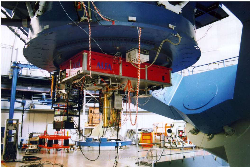
Figure 1.2: The adaptive optics system ALFA attached to the Cassegrain focus of the 3.5-m telescope on Calar Alto. The golden tube below ALFA is the infrared camera Omega-Cass.
