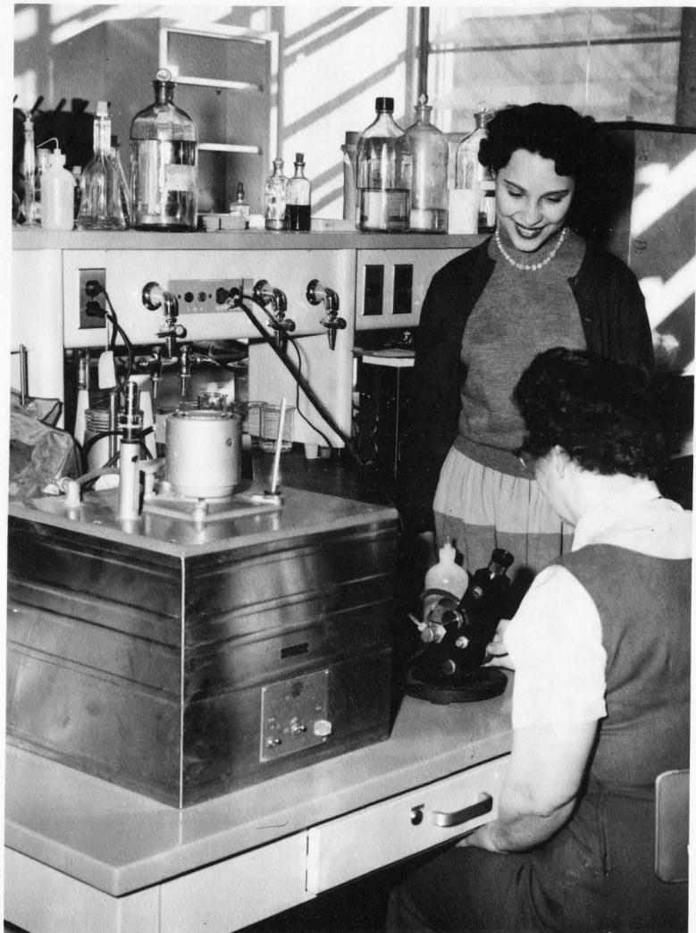
Figure 2. Abbe type refractometer with temperature control attachment
