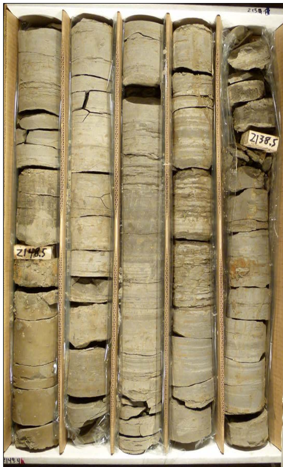
Figure 15. Core box containing mudstone, 829.2 (top right) – 831.2 (bottom left) m bgs. Laminar bedding planes observed, varying in color.
