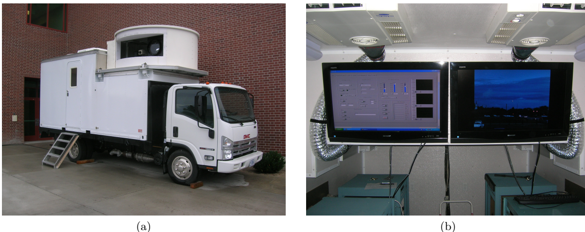
Figure 1: The VISSTA van. (a) The ELT aperture can be seen at the right side in the turret behind the cab. (b) Displays used for system control and display of sensor data.
