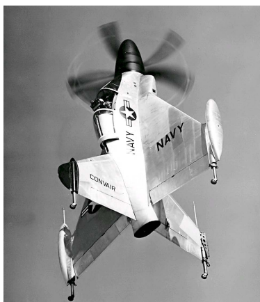
Figure 1. The Convair XFY-1 Pogo in hovering flight.
