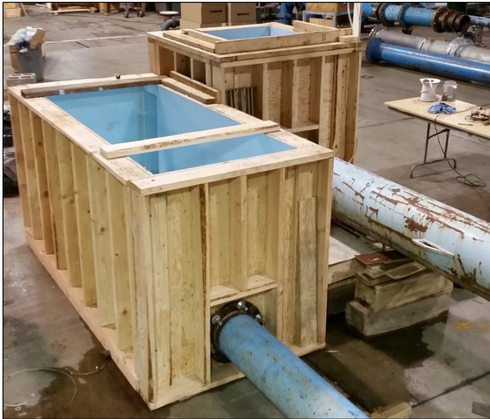
Figure 5. Second box built to collect the flow split.
