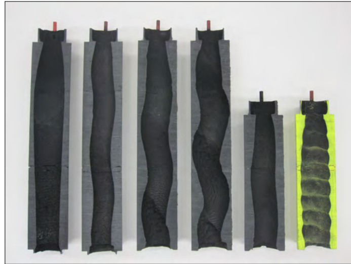
Fig. 4.8: Post-Test Fuel Grain Cross Sections
