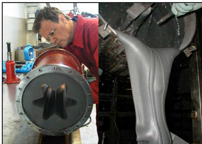
Fig. 1.3: Fuel Grain Manufactured using Cast and Cure Techniques
