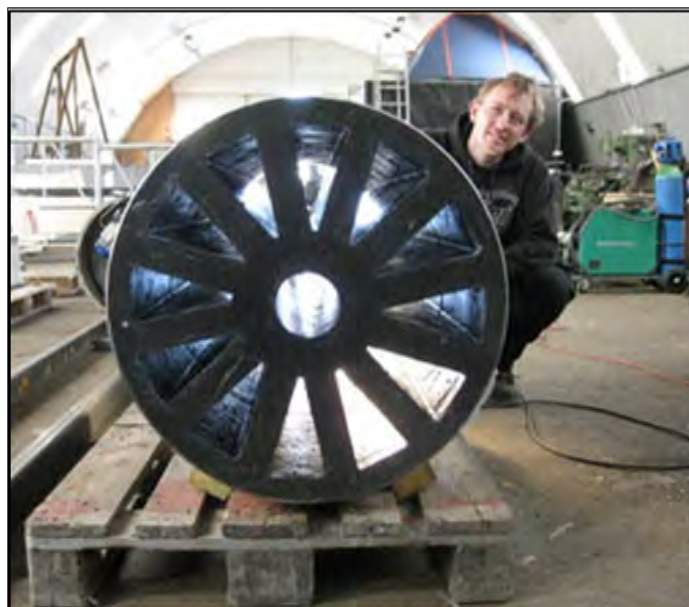
Fig. 1.1: Example of a Multi-Port-Style Fuel Grain
