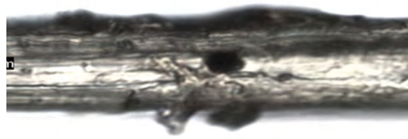
(a) Fiber Delamination
