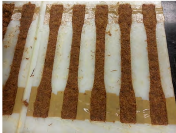
Fig. 3.17: Casting Kenaf Fiber Composite Sample
