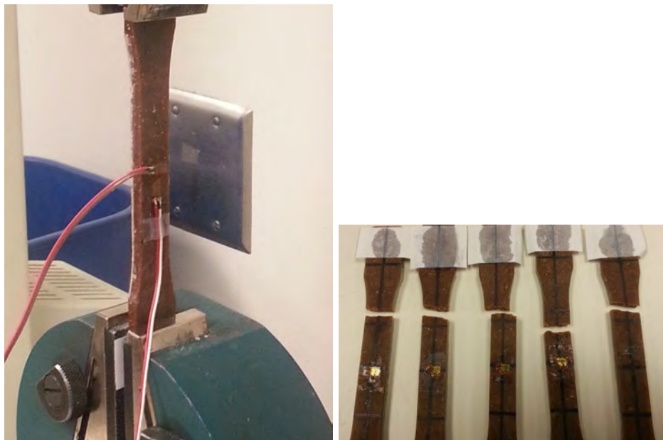
Fig. 3.24: Kenaf Fiber Composite Tensile Test
