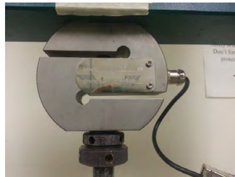
(a) Tinius Olsen Testing Machine Frame (b) Load Cell on Machine Frame
