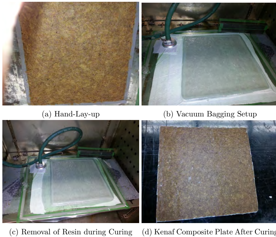
Fig. 3.18: Processing of Kenaf Fiber Composite Plate Using Vacuum Bagging Technique
