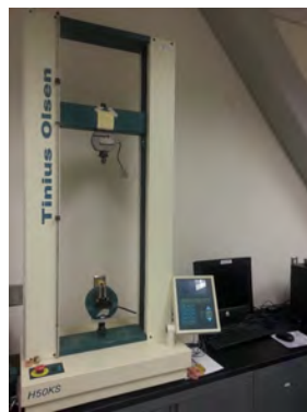
(a) Tinius Olsen Testing Machine Frame (b) Load Cell on Machine Frame
