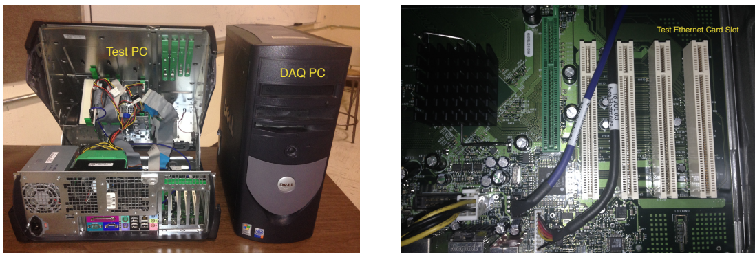
Fig. 2.4: The desktop TPC and DAQPC (left) and the slots of TPC (right).
