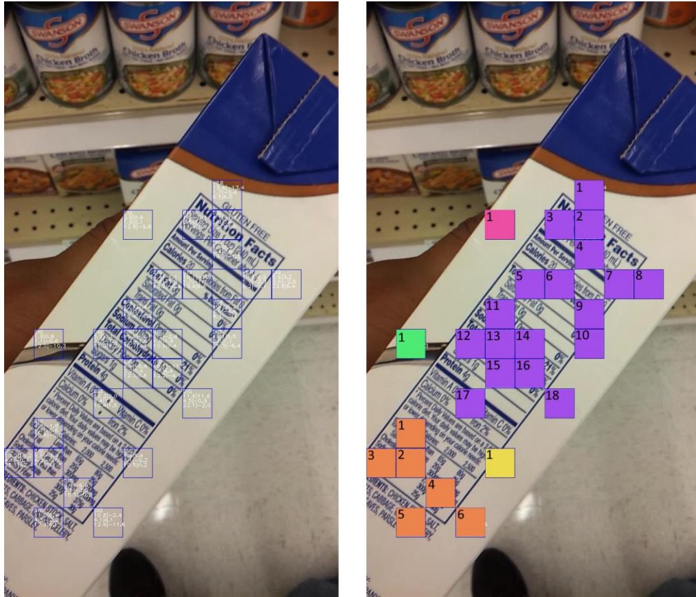
Figure 3.3 Square tiles with pronounced changes (left); Tile clusters found by DFS (right)
