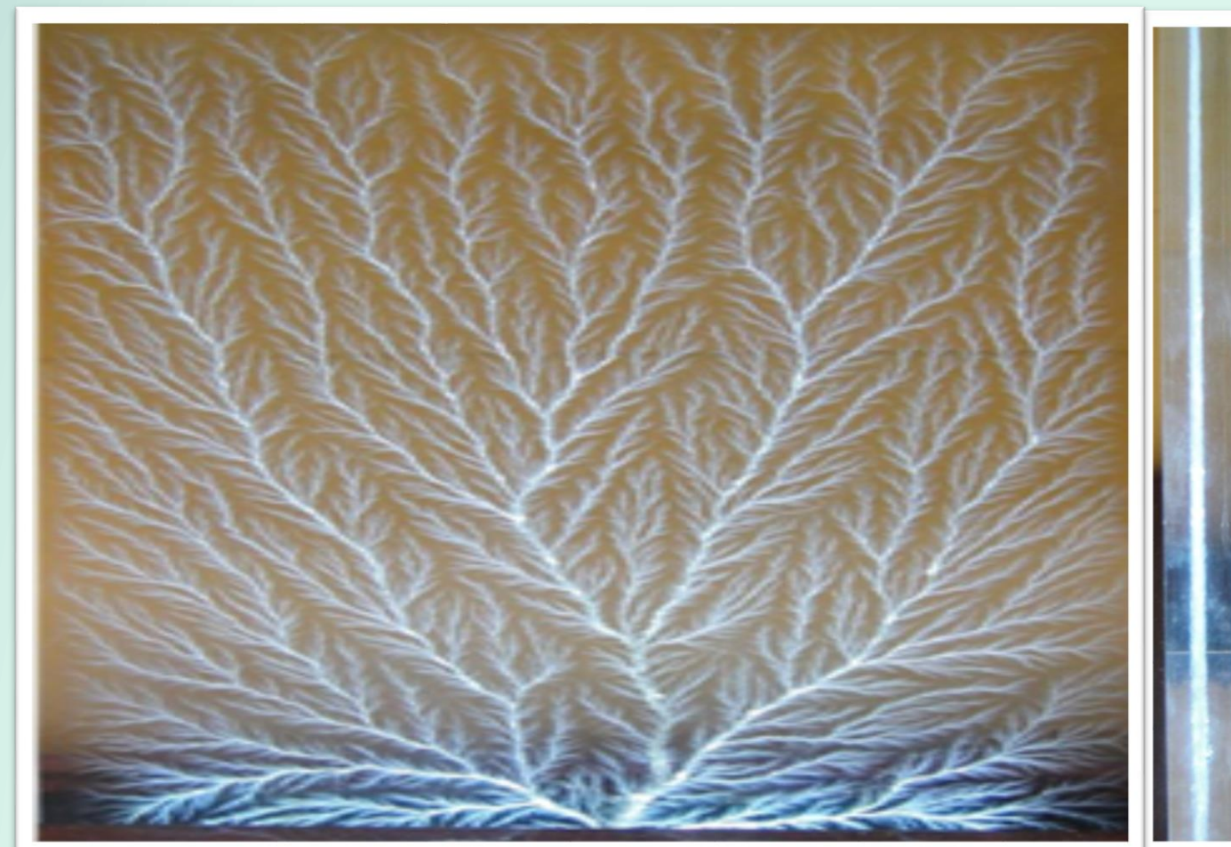
Fig. 1. Front (Left) and side (Right) views of a Lichtenberg discharge tree. The white line (Right) indicates the narrow distribution of deposited charge from a -1 MeV electron beam at R=3 mm in a PMMA sample.
