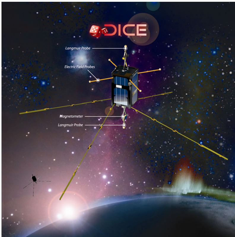
Fig. 2 The DICE mission is a next-generation NSF and NASA-sponsored space research mission formed around CubeSat technologies
