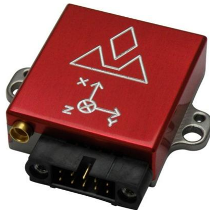
Fig. 6.5: VectorNav VN-200 rugged GPS-aided inertial navigation system
